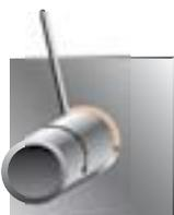
**PB** TUBE EN ROTATION. L'AXE DU TUBE EST HORIZONTAL.
